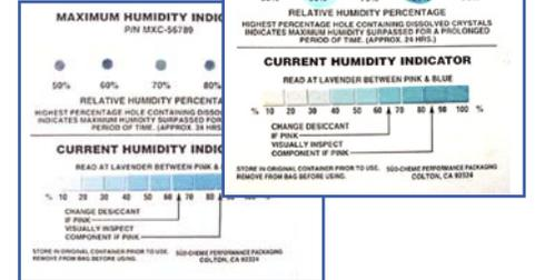
Humitector Maximum Humidity Indicator Cards feature blue crystals that permanently dissolve when a certain humidity level has been reached.
