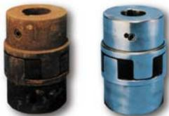
Using Süd-Chemie's Desi Pak<sup>®</sup> or other desiccant bags helps reduce the effects of moisture, such as the rusting of metal parts, shown above.
